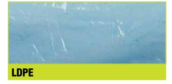
Low Density Polyethylene (LDPE) is the low density version of PE. Similar to PE, LDPE has excellent resistance to water, moisture and most organic solvents and chemicals. LDPE has high ductility but low tensile strength, which is evident by its propensity to stretch. LDPE is highly flexible and perfect for protective garments which have a short term requirement.
